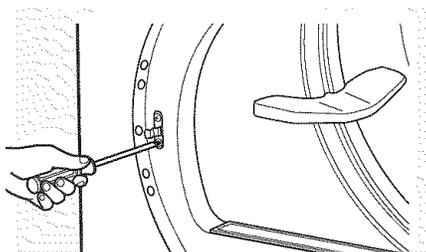
**22.** Switch the strike bracket and its cover on the opposite side by removing the screws; then reinstall both on the opposite side.
