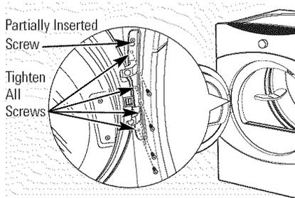
**23.** The door is now ready to be installed on the dryer. To ease this step, the hinge has keyholes that allow a partially fastened screw to be used as a hook.
