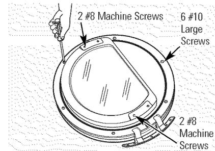
5. Remove the 6 large tapping screws (#10) located around the perimeter of the door outlining the gasket, and the 2 machine screws (#8) on the hinge side.
