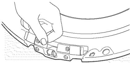
**15.** Place the hinge cover in position. Align the hinge cover holes with the holes in the door.
