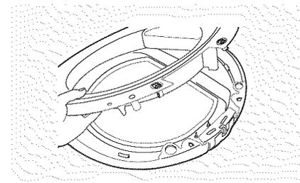
**17.** Place the plastic cover onto the inner door and lock in place with the 4 tabs.
