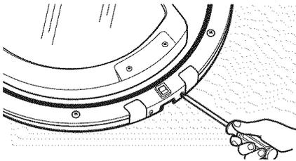
**16.** Secure the hinge cover with the 2 tapping screws (#8).
