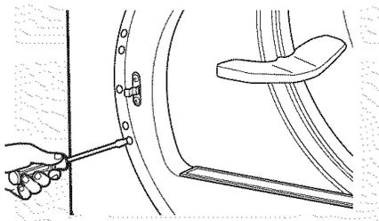
**21.** Using a putty knife or any other flat tool, remove the 5 plastic screw caps located on the dryer where the door will be installed and install them on the opposite side.
