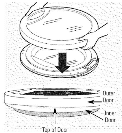
**18.** Place the outer door onto the inner door.
