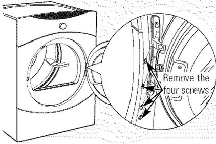
2. Open the door to approximately 90 degrees. Remove the 4 screws starting from the bottom to the top. Make sure the door is supported while removing the screws.
