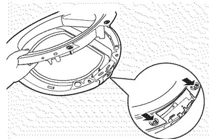
7. Unlock the 4 tabs on the plastic cover and separate the plastic cover from the frame.
