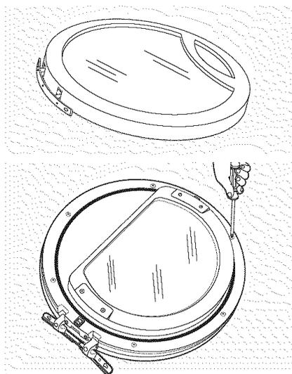
**19.** After reversing door, there will be a mismatch between the outer door and the inner door.
