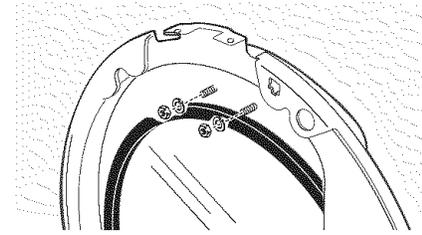
**14.** Place the door on its edge. Assemble the 2 machine screws (#8), washers and nuts. Tighten using a wrench and screwdriver.
