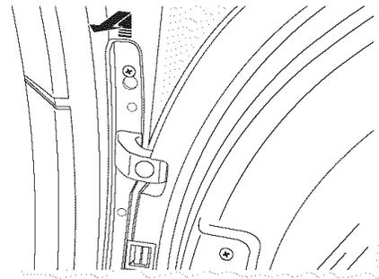
3. Loosen the top screw as shown. Unhook the door by lifting and pulling as shown by the arrows.
