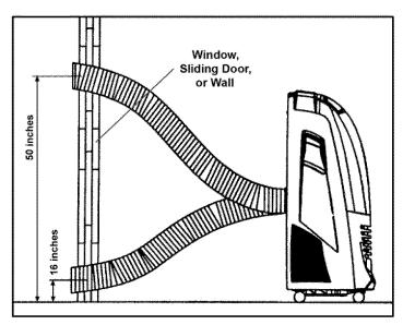
NOTE: In order to achieve maximum room cooling efficiency, the exhaust duct should remain as short and straight as possible. To further shorten the exhaust hose, first unthread either exhaust duct adapter clockwise to remove it. Then cut the hose to desired length. It is not recommended to increase the manufacturer's length of the exhaust hose. This may reduce the cooling efficiency or damage the unit
