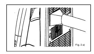
i. Window Kit Mounting: The exhaust hose easily connects to the window kit by snapping the hose adapter directly onto the kit. See page 7 for window/sliding door kit installation.
