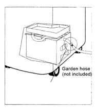
NOTE: When using the continuous drainage method, the unit will NOT shut off automatically when an external water bucket is full. Spill water can cause substantial damages to carpet, floors, furniture and other valuables.
