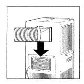
Window Kit Mounting: Connect the window kit adapter to the external end of the exhaust duct. The exhaust duct is now ready to be attached to the window kit. See page 7 for window kit installation
