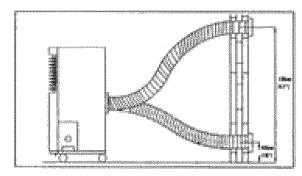
NOTE: In order to achieve maximum room cooling efficiency, the exhaust duct should remain as short and straight as possible. To further shorten the exhaust hose, first unthread either exhaust duct adapter clockwise to remove it. Then cut the hose to desired length. It is not recommended to increase the manufacturer's length of the exhaust hose. This may reduce the cooling efficiency or damage the unit.
