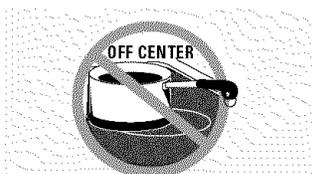
Always center the pan on the surface element you are using.
