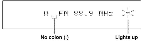
If a colon (:) appears in the front panel display, tuning is not possible. Press PRESET/TUNING to turn the colon (:) off.
