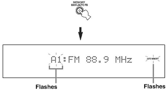
When automatic preset tuning is completed, the front panel display shows the frequency of the last preset station.
