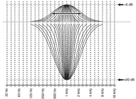
YPAO adjusts frequency characteristics to suit your listening requirements using a combination of the above three parameters (Frequency, Gain and Q factor) for each equalizer band in this unit's parametric equalizer. This unit has 7 equalizer bands for each channel.
