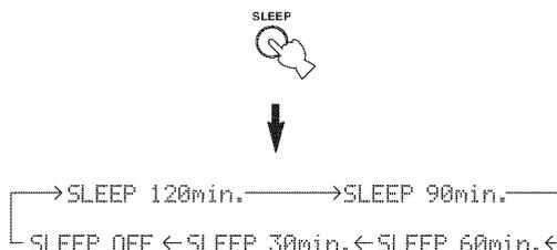
The SLEEP indicator flashes while you are switching the amount of time for the sleep timer. Once the sleep timer is set, the SLEEP indicator lights up in the front panel display, and the display returns to the selected sound field program.
