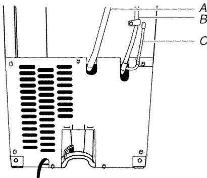
A. Drain hose (drain pump models only)
