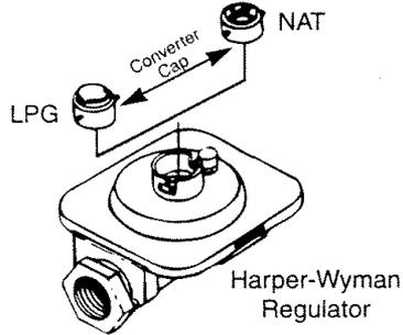
On the SCP regulator, unscrew the converter using a 5/8" wrench. Turn the cap over and reinstall.
