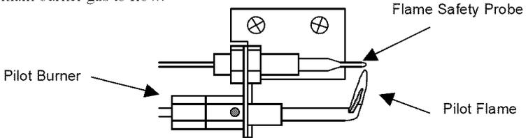
Pilot flame size is set by the adjustment screw located along the side of the thermostat. The outer tip of the flame should just barely reach the underside of the end of the flame safety probe. The pilot screw must be adjusted if the range is converted to LP gas.
