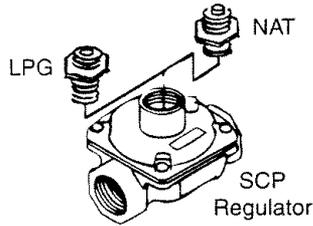
On the Maxitrol regulator, unscrew the brass converter cap using a 7/8" wrench. Turn the selector pin over and re-install.
