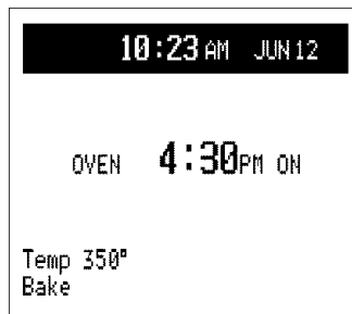
5 If you touch the START pad, the oven will come on at 4:30 PM. If you select Timed Cook (following the directions on page 31) the oven will come on automatically at 4:30 PM, then turn off automatically at the end of the set cooking time.
