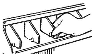
Remove the front grille to adjust the vertical louvers side-to-side to direct the air left or right.
