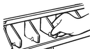
Remove the front grille to adjust the vertical louvers side-to-side to direct the air left or right.
