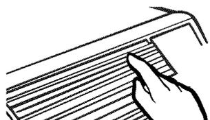
Horizontal louvers on the front grille let you control the air direction up and down.
