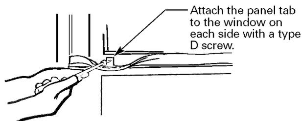
Attach the panel tab to the window on each side with a type D screw.
