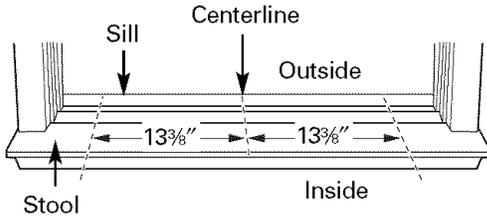
**B** Measure  $12\frac{3}{8}$ " from the centerline on both sides for the sill support brackets.
