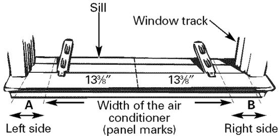
**B** Mark the **A** and **B** measurements on each side of the filler panel board. Cut the panels and discard the center piece. Note position of the notches.
