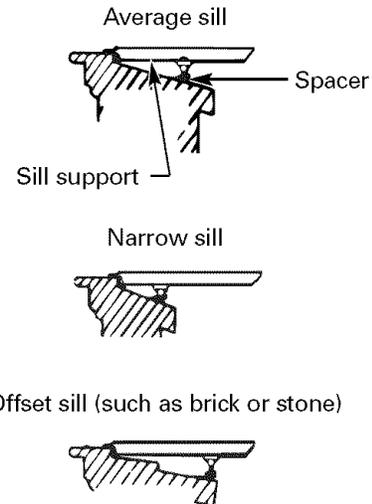
**B** Before attaching the sill supports, place them on the window stool. Select the spacer position that will place the spacer near the outermost point on the sill. Tighten the spacer mounting screws.
