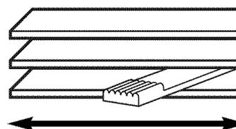
To open the vent, push the lever to the right.
