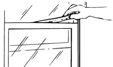
Caulk or weather-strip any gaps or openings to the outside to seal the installation.
