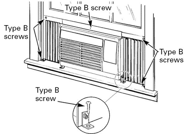
Attach the brackets to the stool on both sides using two type B screws.
