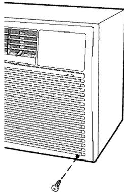
On some models, open the inlet grille from the sides and remove it. Remove the screw from the lower right corner if present.
