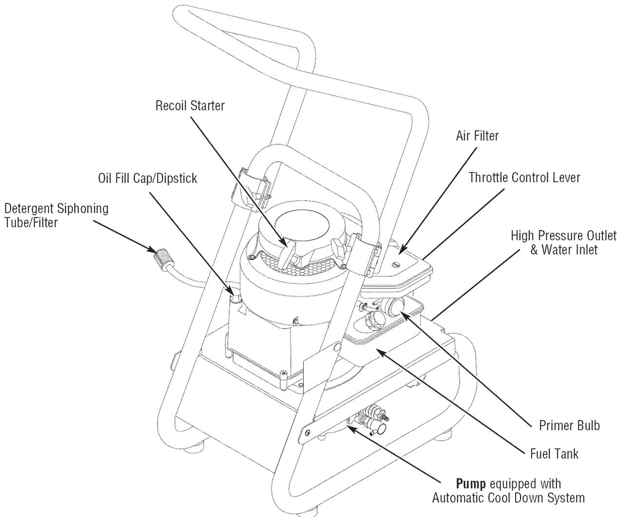
**Air Filter** — Protects engine by filtering dust and debris out of intake air.
