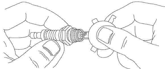
5. Install spark plug, tighten securely.
