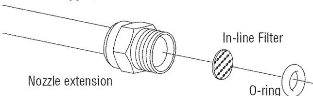
1. Detach nozzle extension from gun and remove o-ring and screen from nozzle extension. Flush screen, gun, and nozzle extension with clean water to clear debris.
