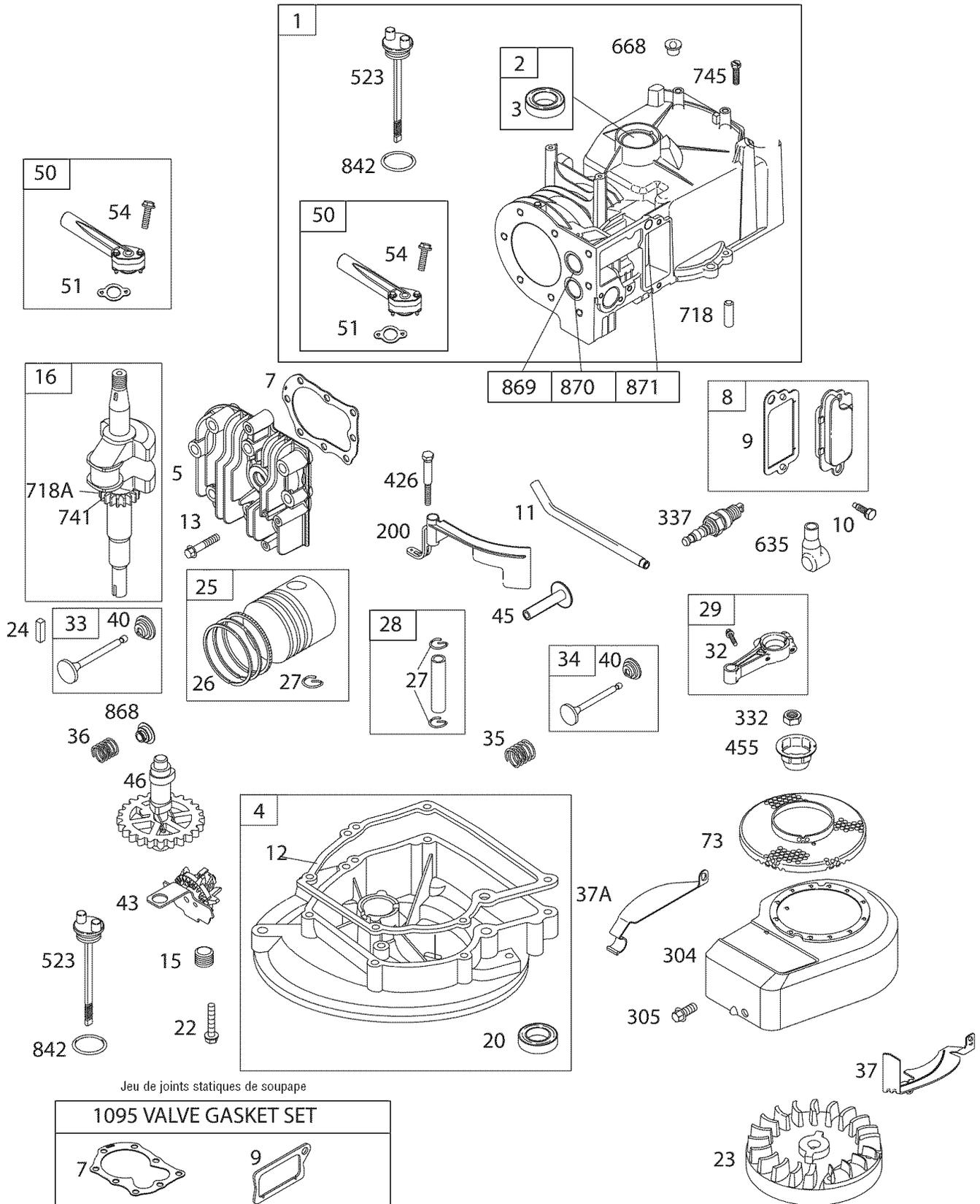
**ENGINE, 3.75 HP, Briggs and Stratton, 9L902 – Exploded View**
