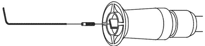
5. Remove in-line filter from other end of nozzle extension.
