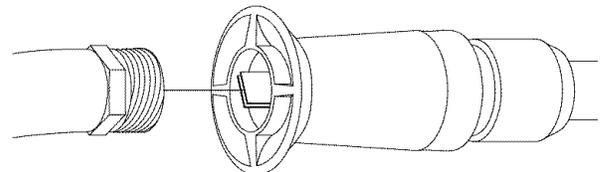
8. Reinstall orifice and in-line filter into nozzle extension. DO NOT overtighten orifice with allen wrench.
