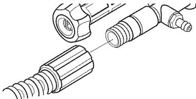
3. Before connecting garden hose to water inlet, inspect inlet screen. Clean screen if it contains debris or have it replaced if damaged. Refer to section "O-Ring Maintenance" if inlet screen is damaged. **DO NOT run pressure washer if inlet screen is damaged.**
