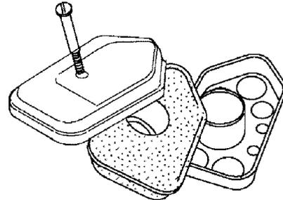
2. Carefully remove air cleaner assembly to prevent debris from falling into carburetor.
