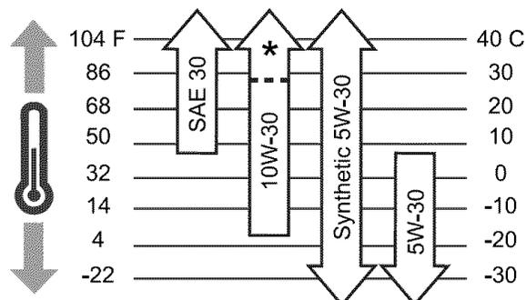
**NOTE:** Synthetic oil meeting ILSAC GF-2, API certification mark and API service symbol with "SJ/CF ENERGY CONSERVING" or higher, is an acceptable oil at all temperatures. Use of synthetic oil does not alter required oil change intervals.
