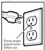
three-prong (grounding) plug which mates with a standard three-prong (grounding) wall receptacle to minimize the possibility of electric shock hazard from this appliance. You should have the wall receptacle and circuit checked by a qualified electrician to make sure the receptacle is properly grounded.
