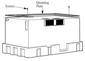
**5** Remove the 2 screws from the mounting plate. This plate will be used as the rear wall template and for mounting. You may discard these screws.
