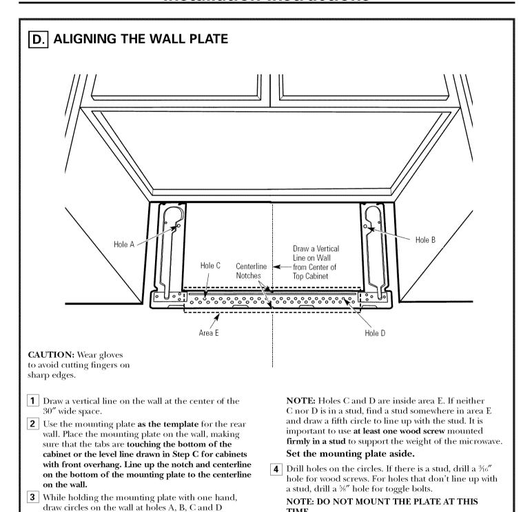
(see illustration above/actual plate marked with arrows). Four holes must be used for mounting. TIME.
