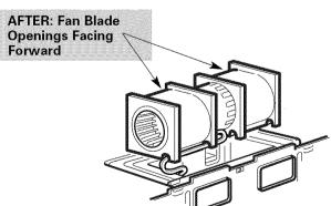
**NOTE:** Make sure wires remain routed in the grooves of the motor frame.
