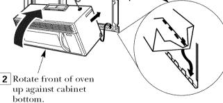
Insert a self-aligning screw through top center cabinet hole. Temporarily secure the oven by turning the screw at least **two full turns** after the threads have engaged. (It will be completely tightened later.) Be sure to keep power cord tight. Be careful not to pinch the cord, especially when mounting flush to bottom of cabinet.
