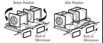
Gently remove the wires from the grooves.
