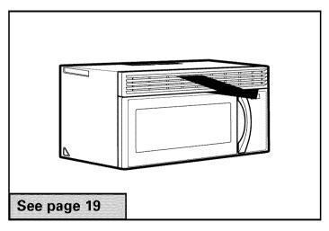
A Charcoal Filter Accessory Kit is required for the nonvented exhaust. (See your Owner's Manual for the kit number.)
