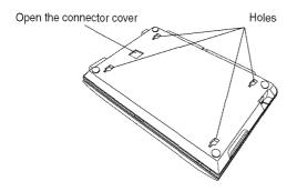
4 Turn the battery pack over and insert the connector hooks into the corresponding holes of the player. ①
