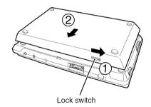
5 Attach the connector cover on the bottom of the player.
