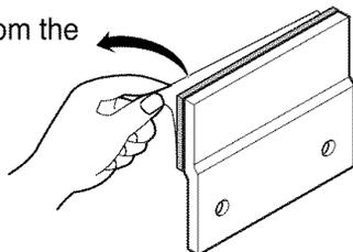
**4** Attach the double-sided tape of the bracket to the dryer as shown so the bent parts of the brackets align with the edge and can be attached to the pedestal with screws.
