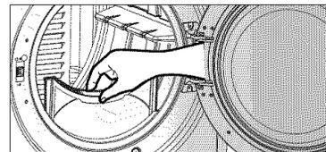
2. Clean the filter using one of the following methods.
