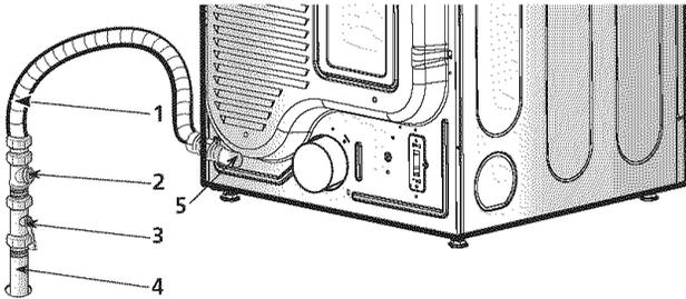
1. New stainless steel flexible connector. Use this type of connector only if allowed by local codes. Use Design AGA Certified Connector.
