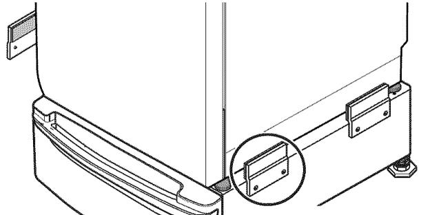
**5** Be sure to press the adhesive parts of the brackets firmly to the appliance.
