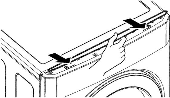
**9** Assemble the upper deco by sliding it down to the left.
