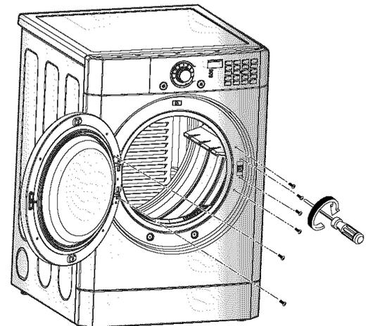
**STEP 3 Procedure of Change Panel****Disassemble**
