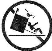
To reduce the risk of tipping, the wall oven must be secured by properly installed anti-tip bracket provided with the wall oven. Refer to the Installation Instructions for proper anti-tip bracket installation.
