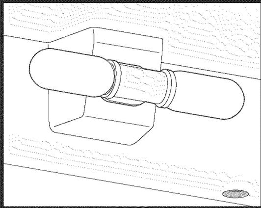
The light comes on automatically when the door is opened. The light bulb assembly is located on the back of the refrigerator control box. To replace the light bulb, turn the temperature control to "OFF" and unplug the electrical cord. Replace the old bulb with a bulb of the same type and wattage.
