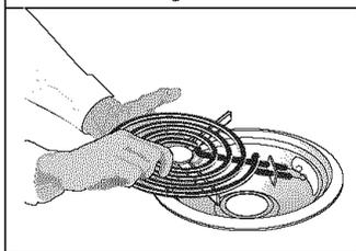
**ATTENTION:** Never leave covers on the coil elements as they could be permanently damaged if the coil is turned on by accident.
