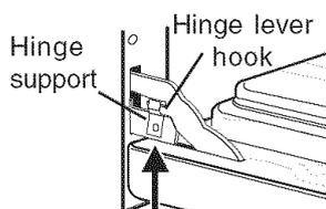
Lock engaged for door removal - Figure 1
