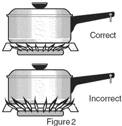
Never extend the flame beyond the outer edge of the utensil. A higher flame simply wastes heat and energy, and increases the risk of being burned by the gas flame.
