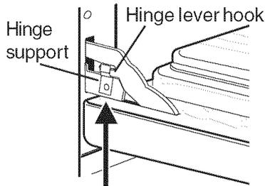
Lock engaged for door removal
