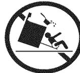
**⚠ WARNING** To reduce the risk of tipping, the range must be secured by properly installed anti-tip bracket(s) provided with the range. To check if the bracket(s) is installed properly, remove the lower panel or storage drawer and verify that the anti-tip bracket(s) is engaged. Refer to the Installation Instructions for proper anti-tip bracket(s) installation.
