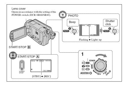
Slide the POWER switch in the direction of the arrow repeatedly until the respective lamp lights up.
