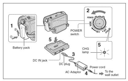
You can charge the battery after attaching the "InfoLITHIUM" battery pack (P series) to your camcorder.
