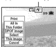
The camera is set to playback mode, then an image and the print menu appear on the screen.
