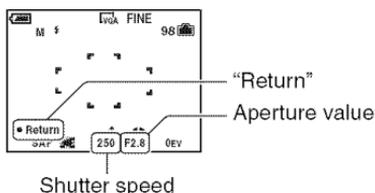
When the zoom is set fully to the W side, you can select an aperture, F2.8 or F5.6.
