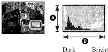
A histogram is a graph showing the brightness of an image. Set the mode dial to P or Scene in advance, then press
