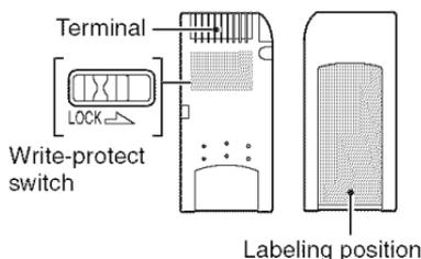
The position and/or the shape of the write-protect switch may differ depending on the "Memory Stick" you use.
