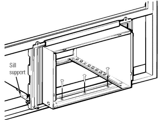
**NOTE:** Do not shut the window so tightly that movement of the accordion panels is restricted.
