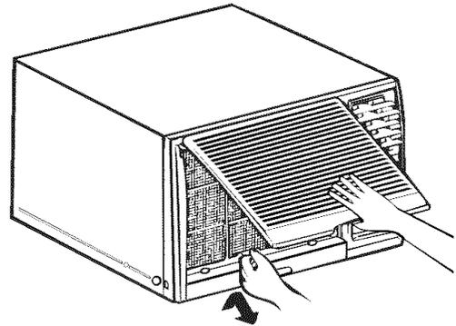
Clean the filter with warm, soapy water. Rinse and let the filter dry before replacing it.
