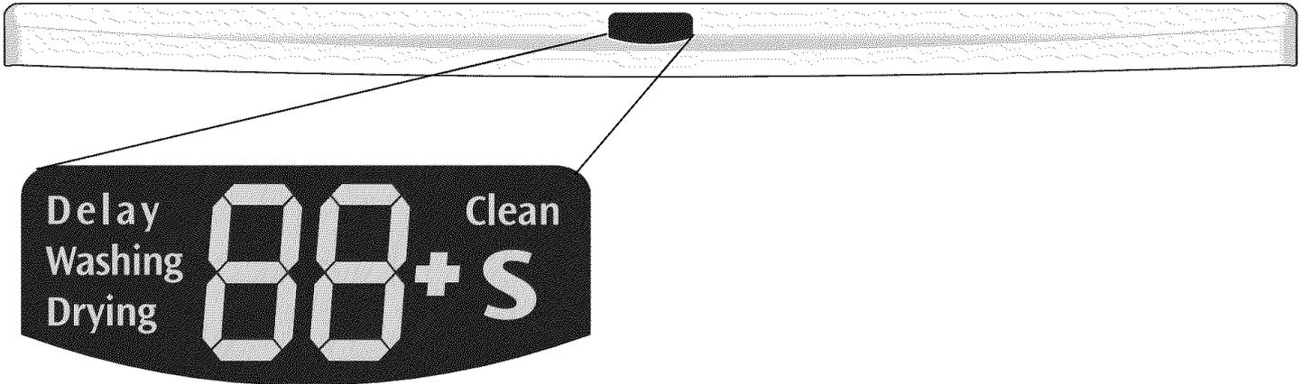
The WASHING light comes on at the beginning of cycle and remains on until the end of the main wash.
