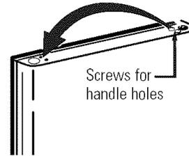
Remove the plug button from the left edge of the door and insert it into the hole on the opposite side.
