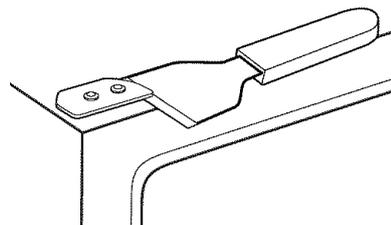
Reassemble the top hinge and shim on the left side, turning the screws just enough to hold the hinge in place.
