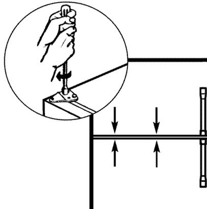
Install the hinge cover over the top hinge.
