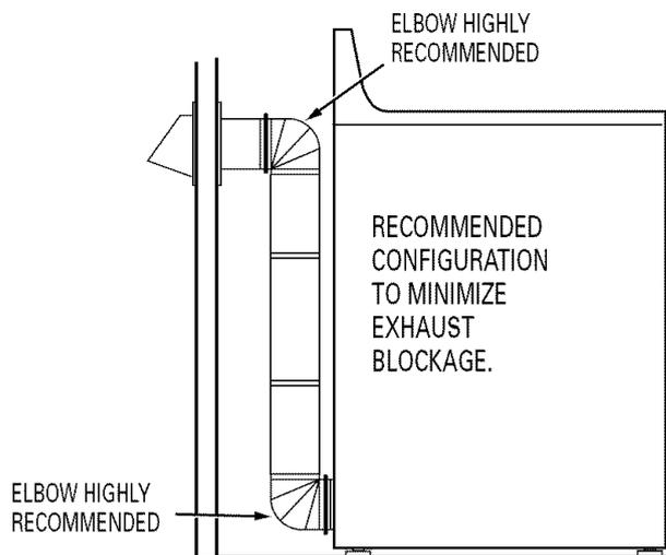
**NOTE: ELBOWS WILL PREVENT DUCT KINKING AND COLLAPSING.**
