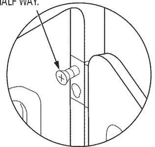
MOVE THE DOOR IN AND DOWN UNTIL THE TOP HINGE AND THE BOTTOM HINGE ARE RESTING ON THE TOP SCREWS INSERTED IN STEP 1.
