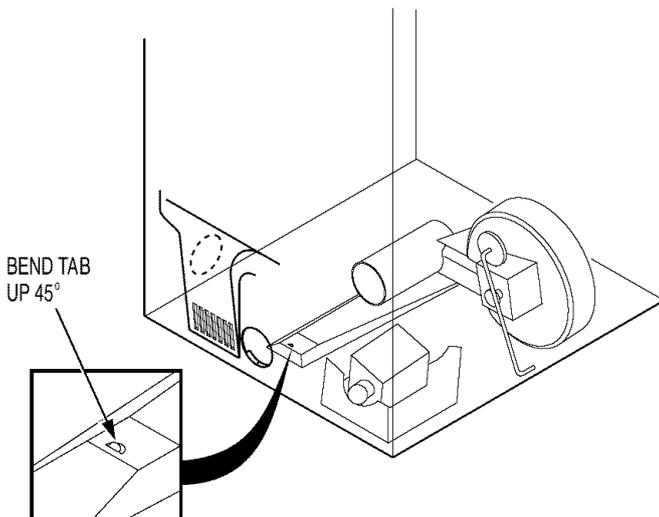
Through the rear opening, locate the tab in the middle of the appliance base. Lift the tab to about 45° using a flat blade screwdriver
