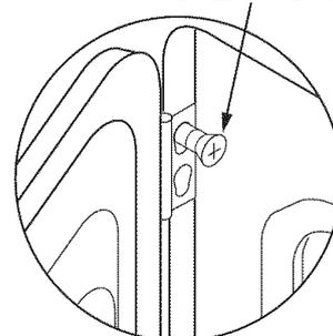
SECURE EACH HINGE AT THE BOTTOM AND TIGHTEN THE TWO TOP SCREWS OF EACH HINGE.
