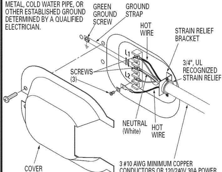
3 #10 AWG MINIMUM COPPER CONDUCTORS OR 120/240V 30A POWER SUPPLY CORD KIT MARKED FOR USE WITH DRYERS & PROVIDED WITH CLOSED LOOP OR SPADE TERMINALS WITH UPTURNED ENDS (NOT SUPPLIED).
