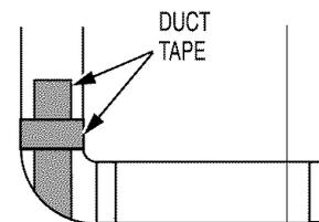
**CAUTION: Internal duct joints must be secured with tape, otherwise they may separate and cause a safety hazard.**
