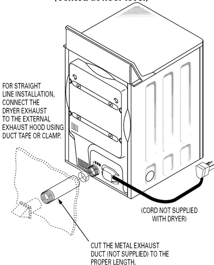
**NOTE: WE STRONGLY RECOMMEND SOLID METAL EXHAUST DUCTING. HOWEVER, IF FLEXIBLE DUCTING IS USED IT MUST BE METAL NOT PLASTIC.**
