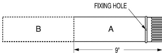
Cut the duct as shown and keep portion A.
