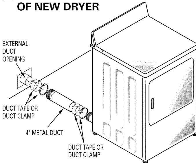
**TIP:** Install your dryer before installing your washer. This will allow better access when installing dryer exhaust.
