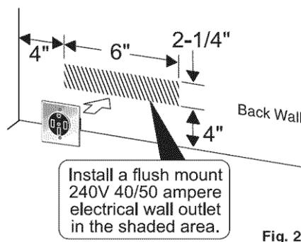
Install a flush mount 240V 40/50 ampere electrical wall outlet in the shaded area.
