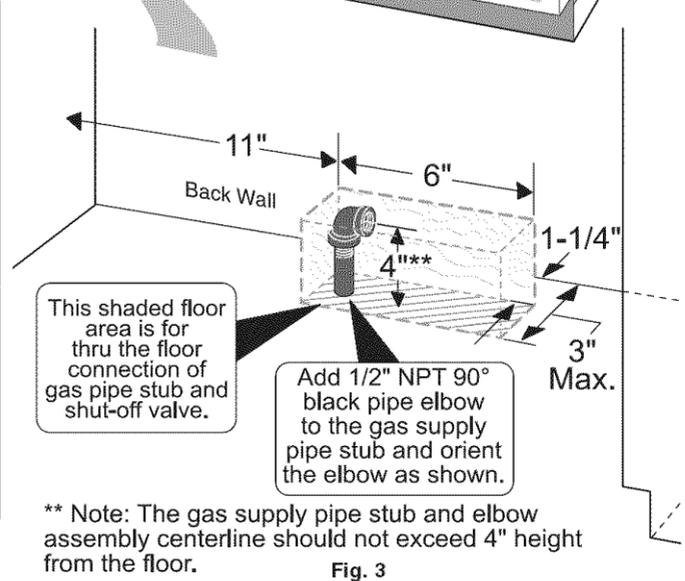
This shaded floor area is for thru the floor connection of gas pipe stub and shut-off valve.
