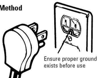
The power cord of this appliance is equipped with a 3-prong (grounding) plug which mates with a standard three-prong grounding wall receptacle to minimize the possibility of electric shock hazard from this appliance.
