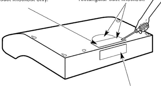
**3/4" x 10" Rectangular horizontal discharge.** Remove rear rectangular duct knockout only.
