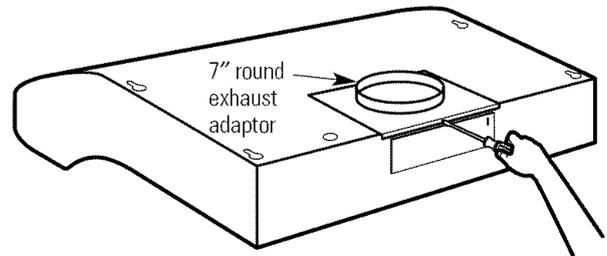
**NOTE:** The 7" round exhaust adaptor can be installed up to 1 inch on either side of the hood center to accommodate off-center ductwork. In extreme off-center installations, one end of the duct connector may need to be trimmed to clear the electrical cable clamp.
