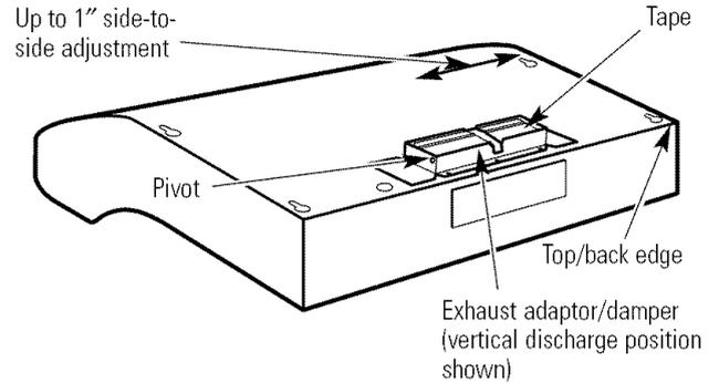
**NOTE:** The exhaust adaptor/damper can be installed up to 1 inch on either side of the hood center to accommodate off-center ductwork. In extreme off-center installations, one end of the duct connector may need to be trimmed to clear the electrical cable clamp.
