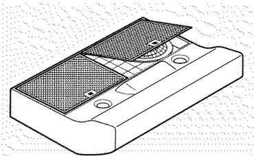
The charcoal filters are clipped inside of each reusable metal grease filter.
