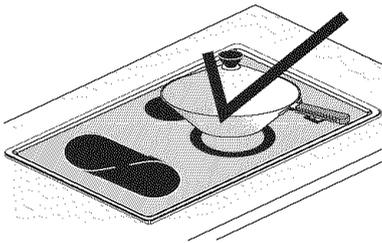
**CAUTION DO NOT** use a wok if it is equipped with a metal ring that extends beyond the surface element. Because this ring traps heat, the surface element and cooktop surface could be damaged.
