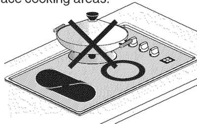
**CAUTION DO NOT** use two surface cooking areas, if your appliance is not equipped with a bridge element, to heat one large pan such as a roaster or griddle. **DO NOT** allow cooking utensils to boil dry. Either of these situations could damage the glass ceramic cooktop.
