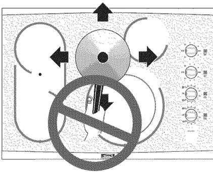
Sliding aluminum or copper clad bottom pans on the cooktop can cause metal markings on the cooktop surface. These marks should be removed **immediately** after the cooktop has cooled using the cooktop cleaning cream. Metal marks can become permanent if not removed prior to future use.
