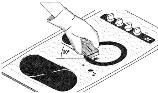
If soils remain, carefully scrape soils with a metal razor blade scraper, holding scraper at a 30 degree angle to the surface. Remove loosened soils with cooktop cleaning cream and buff surface clean.
