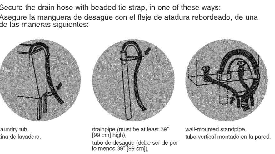
Secure the drain hose with beaded tie strap, in one of these ways:
