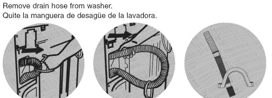
Locate the pull tie to remove drain hose from washer. Pull drain hose straight out of washer by first grabbing the pull tie.
