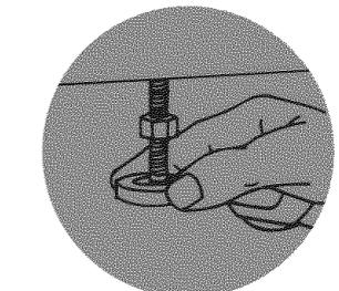
Push on the upper front panel to be sure that the washer is on the rear feet.
