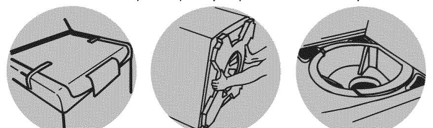
Lid must be taped in place prior to moving the washer.
