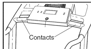
To measure your heart rate, **stand on the foot rails** and hold the metal contacts on the handrail—**avoid moving your hands**. When your pulse is detected, the heart symbol in the display will flash each time your heart beats, one or two dashes will appear, and then your heart rate will be shown. **For the most accurate heart rate reading, continue to hold the contacts for about 15 seconds.**
