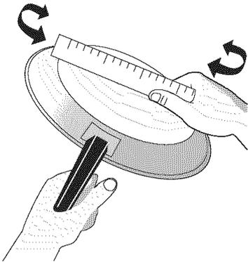
Cookware should have flat bottoms that make good contact with the entire surface heating element. Check for flatness by rotating a ruler across the bottom of cookware. Be sure to follow the recommendations for using cookware that has shown in the illustration at right.
