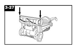
Raise nozzle up and replace the 2 screws on the bottom.
