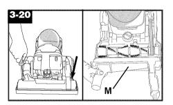
Remove the 2 screws behind the agitator cover.
