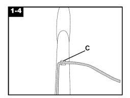
**Cord clip**To help keep the cord out of the way while cleaning, position cord into cord clip (C).
