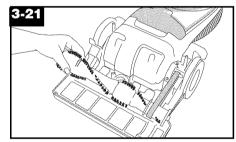
Remove agitator and used belt. Discard used belt.
