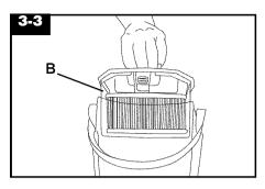
Remove filter chamber (B) from dirt cup.
