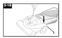
Press on handle release pedal (L) and lower the nozzle so it is flat.
