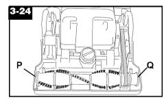
Grasp agitator firmly and fit it into position by first sliding end opposite the belt into the rectangular slot (P) on side of cleaner.
