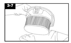
Holding lid, tap bottom of filter against edge of wastebasket until dust particles stop falling from filter.
