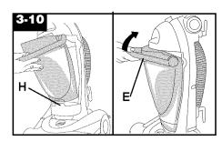
Place bottom of cup behind tab (H) and press cup into cleaner.
