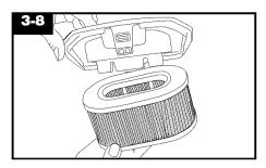
Although not necessary, the filter can be removed from the lid for cleaning.
