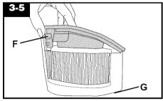
Press latch (F) on front of filter chamber and remove lid. The pleated filter is attached to the lid.
