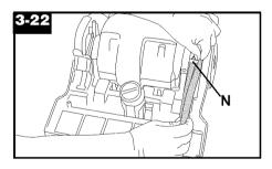
With lettering to the outside of belt, slide new belt along side of cleaner cavity and over motor pulley (N).
