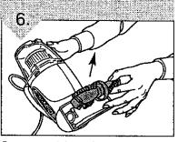
Remove metal nozzle guard and pull brushroll and belt straight out from unit,
