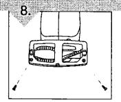
Attach the metal nozzle guard, ensuring that tab is engaged before securing with the screws.
