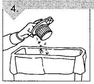
To clean, tap filter assembly against wastebasket to remove remaining dirt and then return filter assembly to dirt cup. If replacing filter, proceed to step 5.
