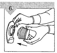
Twist and lock new filter into filter adaptor.
