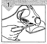
With the unit turned off and unplugged, use a phillips screwdriver to remove the belt door screw located above the brushroll window.
