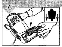
With the new belt properly located in the channel on the middle of the brushroll, slide the brushroll straight down into the unit. **NOTE:** *Make sure the brushroll end caps align with the tabs inside the brushroll housing (see inset).* Brushroll is not symmetrical, its orientation is important.
