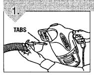
Connect adaptor plate/hose to metal nozzle guard by latching the two longer tabs on the adaptor plate with the rear of the nozzle guard. Pivot the adaptor plate/ hose upward to latch the two smaller tabs on the adaptor plate with the front of the nozzle guard.
