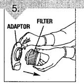
Twist old filter to remove from filter adaptor. **IMPORTANT:** DO NOT DISCARD FILTER ADAPTOR.
