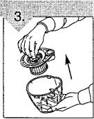
Grasp center tab on filter adapter. Pull out of dirt cup to remove filter assembly.
