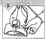
Dip the belt lifter inside the belt access area and hook the belt around the lip of the belt lifter. Slip the belt onto the motor shaft until the belt lifter base meets the shaft. To ensure proper belt placement, gently turn belt lifter counterclockwise and remove. Make sure belt is on shaft.
