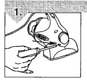
With the unit turned off and unplugged, use a phillips screwdriver to remove the belt door screw located above the brushroll window.
