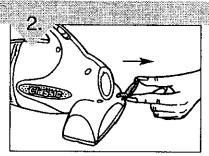
Slide the belt door down and angle out to remove from the unit.
