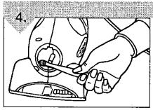
Dip the belt lifter inside the belt access area and hook the belt around the lip of the belt lifter. Slip the belt onto the motor shaft until the belt lifter base meets the shaft. To ensure proper belt placement, gently turn belt lifter counterclockwise and remove. Make sure belt is on shaft.
