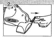
Slide the belt door down and angle out to remove from the unit.
