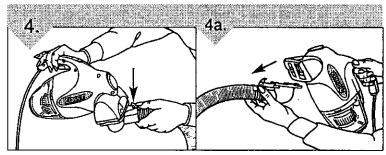
**NOTE:** To remove adaptor plate/hose, push in on the adaptor plate/hose release button while pivoting the adaptor plate down and away from the metal nozzle guard.
