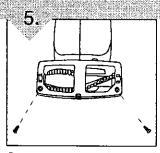
Remove screws on bottom of metal nozzle guard as shown.
