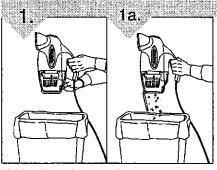
Hold unit as shown and press the dirt cup release button to empty contents into wastebasket. **NOTE:** For best results, periodically remove filter and tap against wastebasket to remove remaining dirt.
