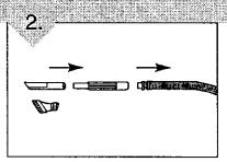
With adaptor plate/hose connected to the metal nozzle guard, select the appropriate tool or combination of tools to attach to the end of the hose. 3.
