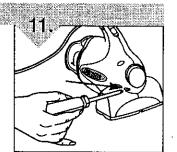
Attach belt door to unit and secure with screw.
