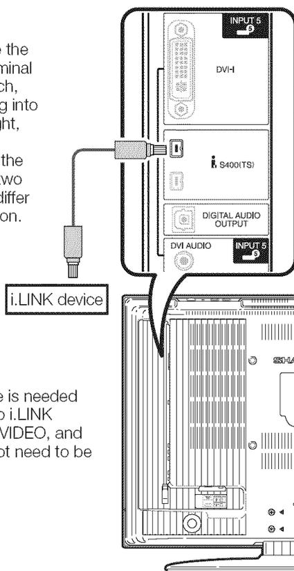
Only an i.LINK cable is needed to connect the TV to i.LINK devices. (VIDEO, S-VIDEO, and AUDIO cables do not need to be connected.)
