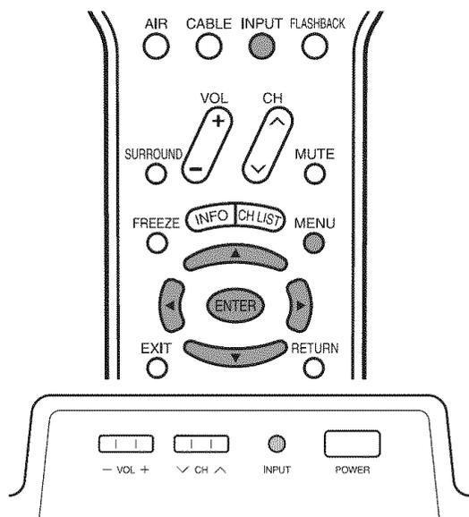
To watch a DVD image, select "INPUT1" from "INPUT SOURCE" menu using **INPUT** on the remote control unit or on the TV. (See page 47.)
