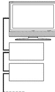
When 3 or more i.LINK devices are connected, branch connection can be used. With branch connections, up to 62 i.LINK devices can be connected.
