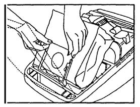
3. Form new bag into a box-like shape. Slide bag collar firmly into holder.
