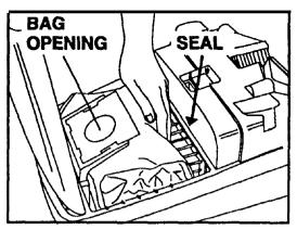
4. Push rear edge of bag into bag cavity below seal.
