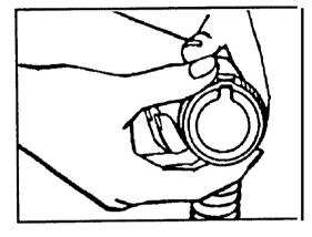
Push hand grip down onto wand or tool so that button projection fits into slot. Turn latch ring to lock in place.
