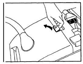
1. Rotate hose to the side, lift bag lid latch and open bag lid.
