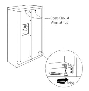
**NOTE:** A nylon plug is imbedded in the threads of the pin. The plug is designed to prevent the pin from turning. A wrench must be used to turn the pin.
