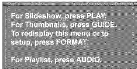
Figure 6. Media dialog box, slide show mode. A similar dialog box appears when in audio mode.
