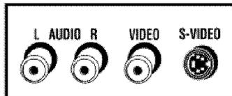
**S-VIDEO (INPUT)** Lets you connect external devices which have S-Video outputs such as:
