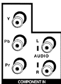
**COMPONENT IN** Lets you connect devices which have component (Y Pb Pr) outputs such as VCRs, DVD players, DVD-PVRs, DVD recorders, satellite receivers and cable boxes. This connection provides optimum picture quality because the video is separated into three signals. Use the AUDIO L and R jacks from the VIDEO IN input to connect for sound.
