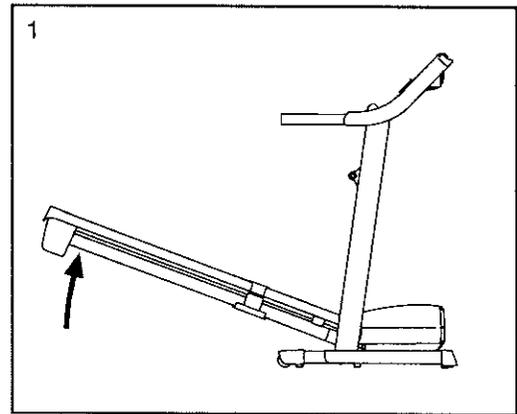
2. Move your right hand to the position shown, and hold the treadmill firmly. Using your left hand, pull the latch knob to the left and hold it. Raise the frame until the catch is past the latch pin. Then, slowly release the latch knob. **Make sure that the frame is securely held by the latch pin.**
