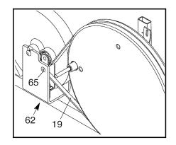
the Flat Head Screw. Then, reattach the side shields.
