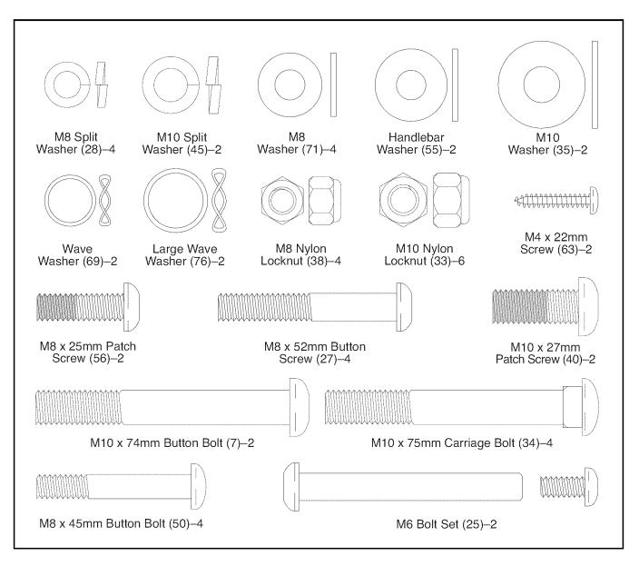
Identify the Stabilizer (9) which has round Endcaps (21) on the ends. While another person lifts the front of the Frame (1), attach the Stabilizer to the Frame with two M10 x 75mm Carriage Bolts (34) and two M10 Nylon Locknuts (33).
