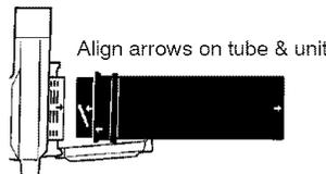
4. To attach the lower vacuum tube to the upper vacuum tube, first align the arrows on the two tubes. Then, press the two tubes together until the lower tube is securely seated in the upper tube (about 3 inches).
