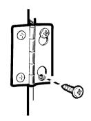
Remove the remaining screws from the side of the opening from which the door was removed. With these screws secure each hinge at the bottom. Tighten the two top screws of each hinge. Reinsert the plastic plugs on the side from which the door was removed.
