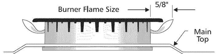
Adjust flame until you can quickly turn knob from LITE to LOWEST POSITION without extinguishing the flame. Flame should be as small as possible without going out.
