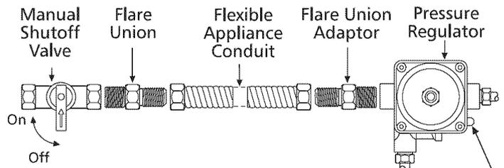
Service Shut-Off Valve Electric Ignition models only
