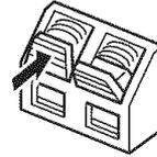
**3** Insert one of the AM loop antenna lead wires into the AM ANT terminal.
