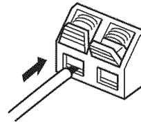
**4** Release the tab of the AM ANT terminal back into place.
