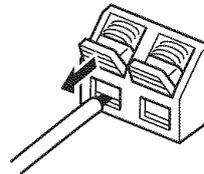
**5** Repeat steps 2 through 4 to connect the other lead wire to the GND terminal.
