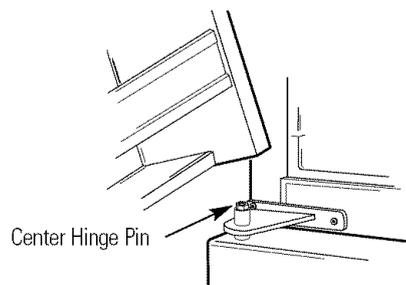
Lift the top hinge so the pin fits into the door socket.
