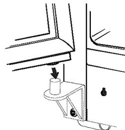
Straighten the door and line it up with the center hinge bracket.
