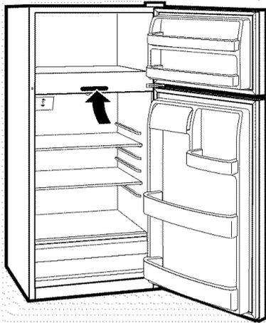
The temperature controls are preset in the factory at **37°F** for the refrigerator compartment and **0°F** for the freezer compartment. Allow 24 hours for the temperature to stabilize to the preset recommended settings.
