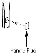
Remove the two screws holding the handle to the top of the door.
