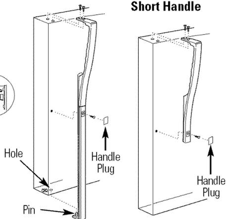
**After removing the handle:** Move the small plug buttons from the top right side of the door top and insert them into the holes on the opposite side.
