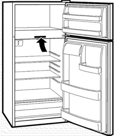
Initially, set the refrigerator control at **5** and the freezer control at **5** and allow 12–24 hours for the temperature to stabilize.
