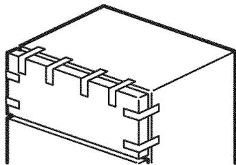
Remove the hinge cover on top of the freezer door (on some models).
