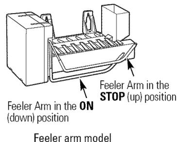
**NOTE:** In lower water pressure conditions, the water valve may turn on up to 3 times to deliver enough water to the icemaker.
