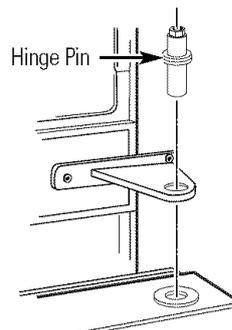
Remove the tape and tilt the door away from the cabinet. Lift the door straight off the bottom hinge bracket.
