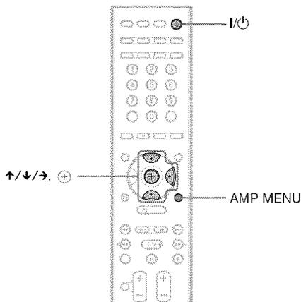
After connecting the AC power cord (mains lead), the demonstration appears in the front panel display. When you press I/⏻ on the remote, the demonstration turns off.
