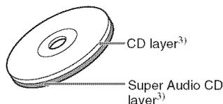
A Super Audio CD layer consists of the 2 channel area or the multi-channel area.
