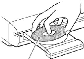
When you play an 8 cm disc, place it on the inner circle of the tray. Be careful that the disc is not skewed on the inner circle of the tray.
