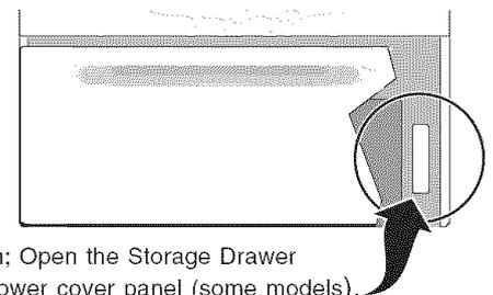
Serial plate location; Open the Storage Drawer (some models) or lower cover panel (some models).
