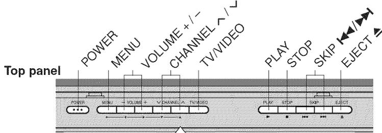
The volume and channel buttons on the top panel can be used as ▲/▼ and ◀▶ buttons while the TV menu is displayed on screen.
