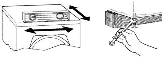
If the washer is against a wall, move the washer out slightly before tipping back. First prop the front with a wood block and adjust the feet as necessary; then prop the back and adjust feet as necessary. Repeat this step until washer is level.
